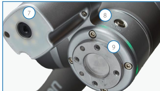
7. Built-in camera with integrated light
