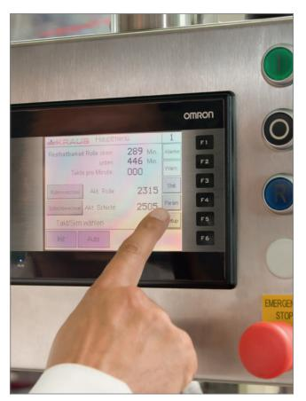
Omron has helped Kraus Maschinenbau to create a solution that adds serialisation capabilities to its printed code inspection system. The inspection tool is part of a friction feeder on an e-cigarette packaging line. The addition of this serialisation capability allows for the printing and verification of a unique code onto each package.
