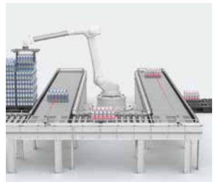
Detecting an accumulated shrink-wrapped pack of bottles
