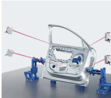
Identifying the vehicle model from the body panel
