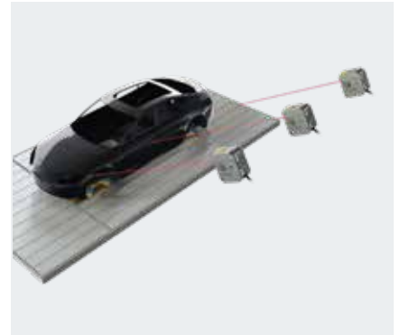
Sensing whether a black-painted body is positioned in place
