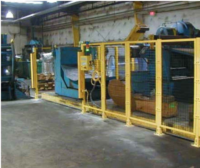
Perimeter guarding system to guard aluminum coil slitting line.
