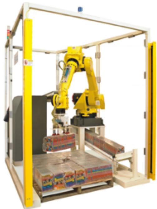
Both conventional and robotic palletizers can receive product at a high elevation (typically between 84" - 2.13m to 124" - 3.15m) or low "floor level" elevation (typically at 30" - 0.76m to 36" - 0.91m). All of these types of palletizers can be part of an automated system or a standalone manual machine.
