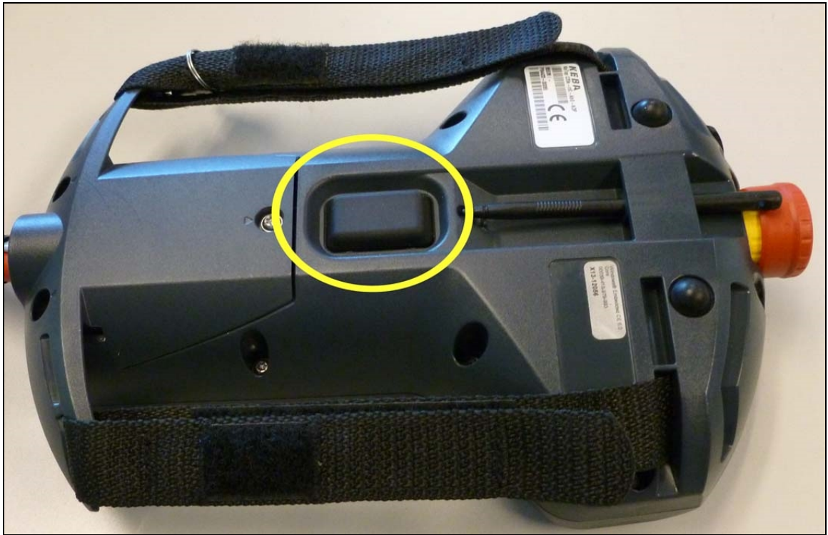
Figure 4-3. 3-Position Enable Switch (Circled)
