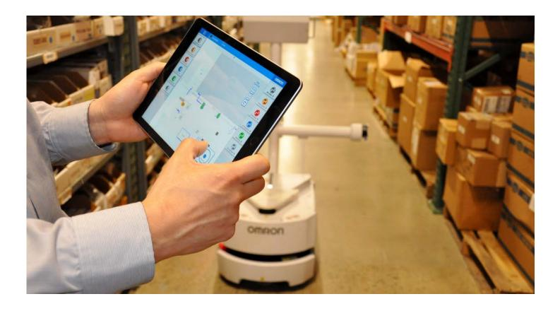
Omron MobilePlanner Tablet Edition is an easy to use, portable, monitoring and control user interface tool for LD mobile robots. The MobilePlanner Tablet Edition is a lite user interface designed for viewing and controlling the robot fleet from a mobile device or tablet.
