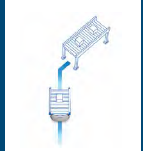
High Accuracy Positioning System (HAPS) HAPS allows our mobile robots to move along fixed paths in applications that require tight tolerances.
