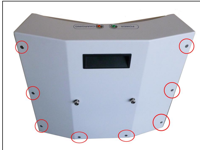
Figure 8-15 Docking Station Rear Cover Screws (8 of 10)
