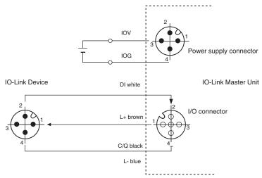
Note: Even if you connect to IO-Link devices without digital inputs for pin 2, connect pin 2 as shown in the above figure. This is because connectors on the IO-Link devices and the cable with connectors on both ends connect pin 2. However, because no data enters pin 2 of the IO-Link Master Unit, digital IO-Link input data is always OFF.
