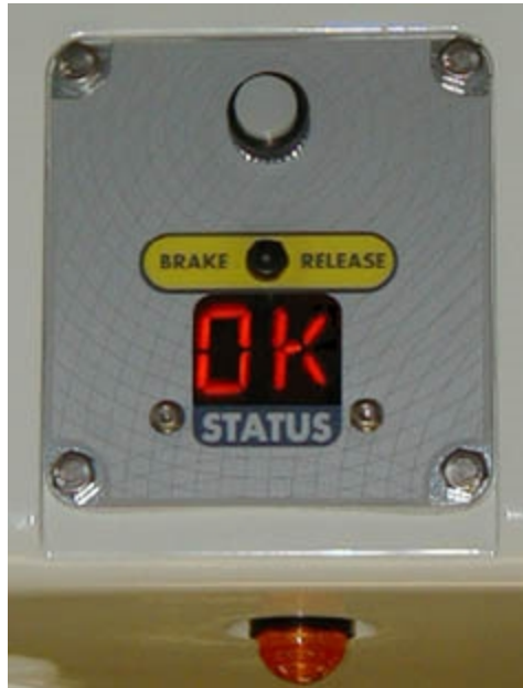
Figure 8-8. Status Display Panel, Showing 4 hex-head Bolts
