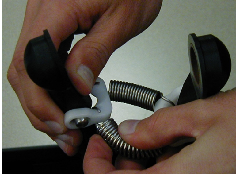
Figure 9-10. Removing an Outer Arm Spring
