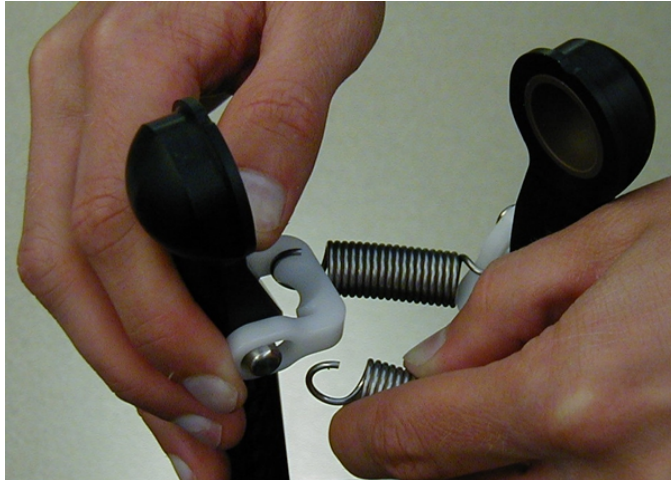
Figure 8-11. Spring, with End Removed from Horseshoe
