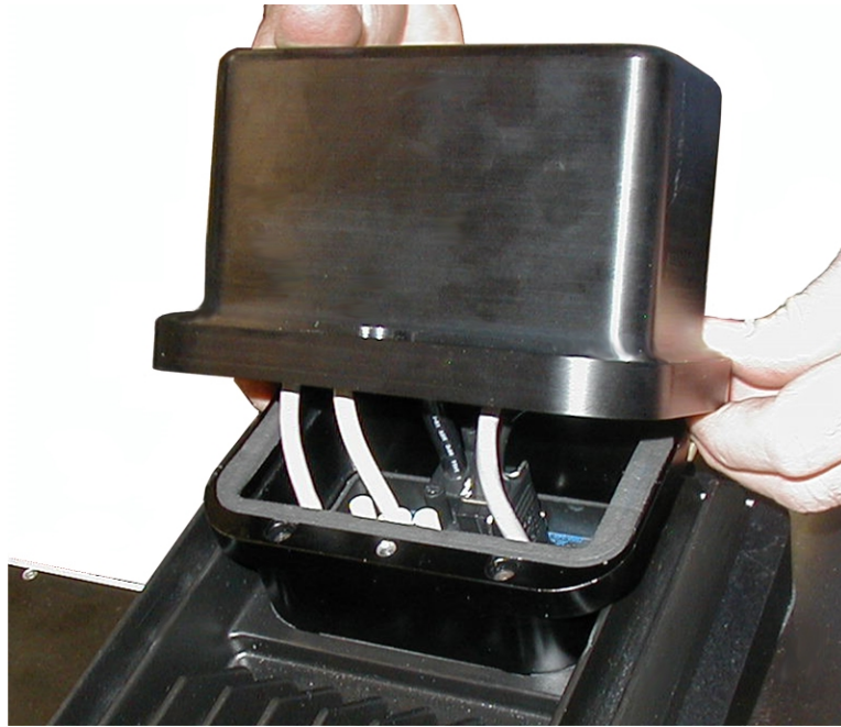
Figure 10-10. Installing Cable Entry Top Cover Assembly
