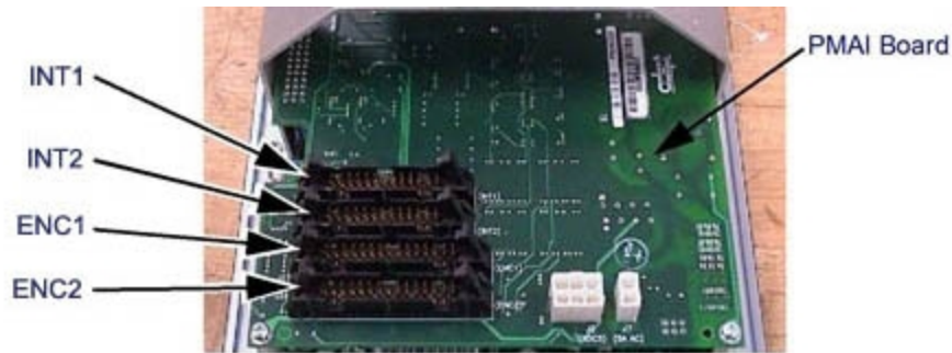
Figure 9-2. Connectors on AIB/eAIB Chassis and PMAI/ePMAI Board (AIB Shown)
