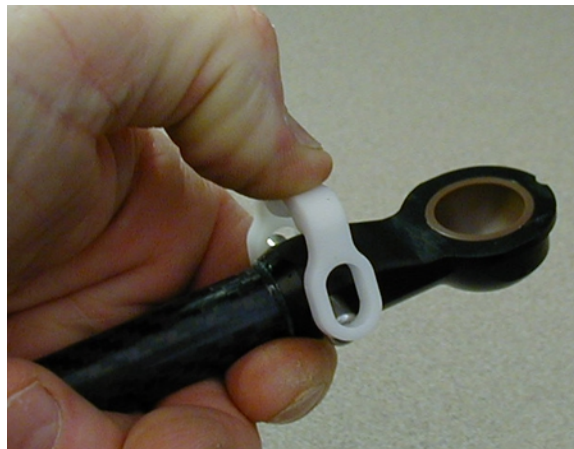
Figure 9-14. Squeezing the Horseshoe into Position
