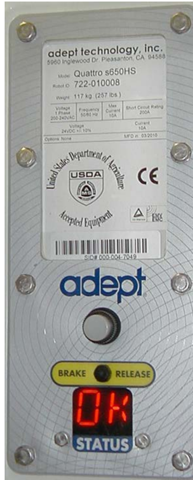
Figure 9-7. Status Display Panel, Showing 8 Hex-head Bolts
