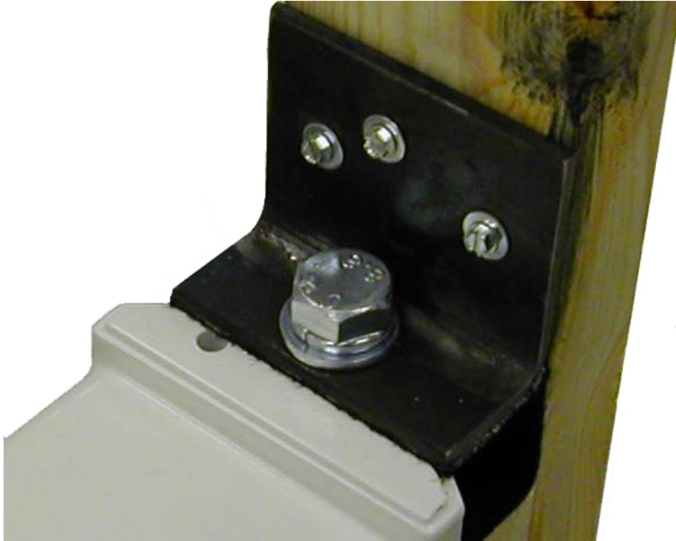
Figure 3-3. L-Bracket Securing Robot to Shipping Crate
