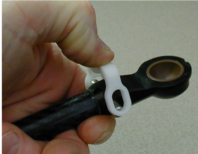
Figure 8-14. Squeezing the Horseshoe into Position
