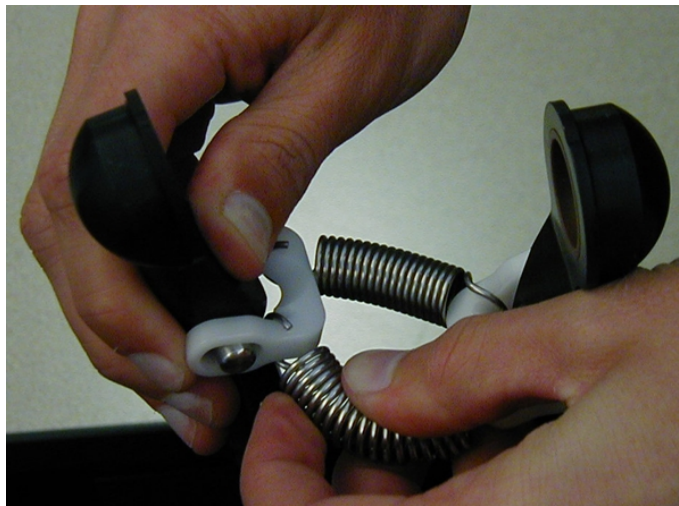
Figure 8-10. Removing an Outer Arm Spring
