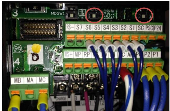
4.) GS1 and GS2 on the MX2 side must be wired into S3 and S4.
