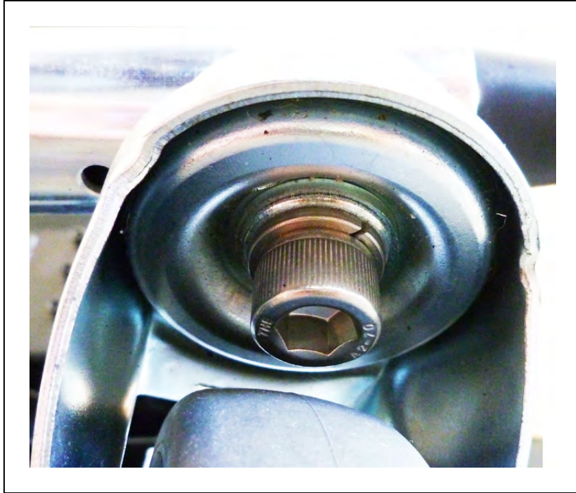
Figure 10-25. Front Cart Caster Screw Assembly
