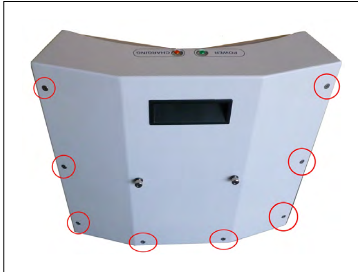
Figure 10-15. Docking Station Rear Cover Screws (8 of 10)
