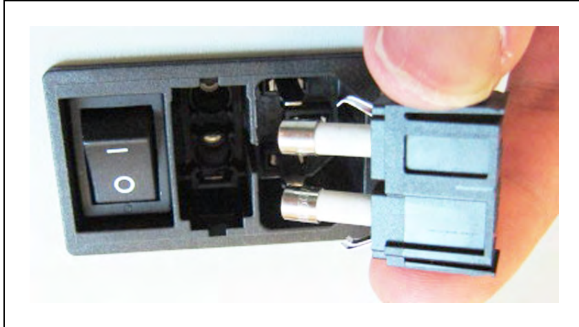
Figure 10-14. Docking Station Fuse
