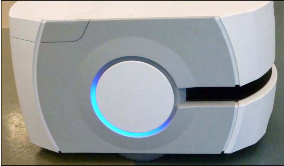
Figure 10-11. Right Side Cover, Showing Even Gaps at Edges
