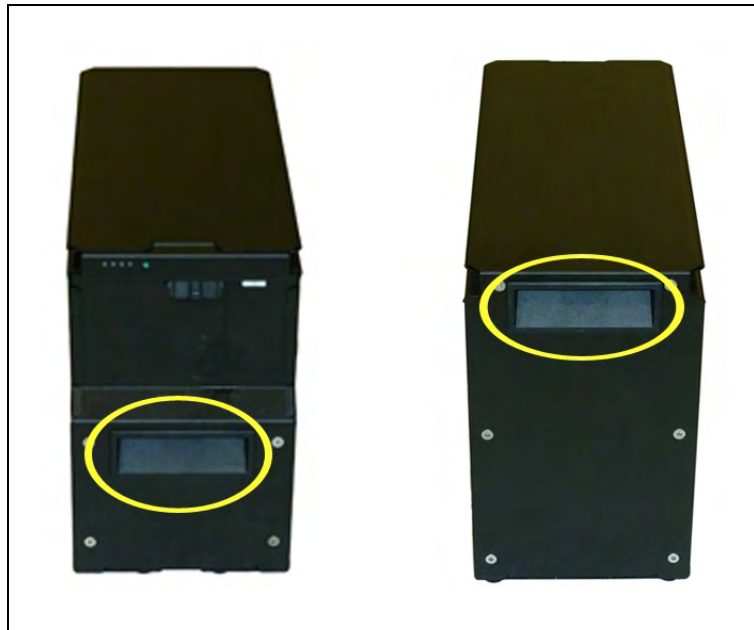
Figure 3-12. Battery Recesses, for Gripping
