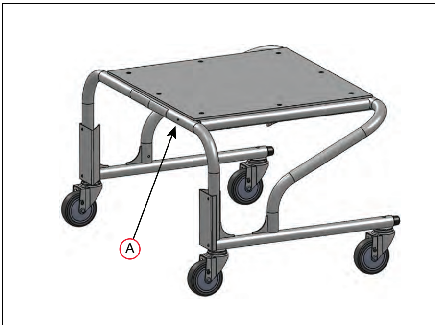
Figure 3-23. Thru-hole for Brake-release Cable, (A) 6 mm diameter (0.25 in.) pass-through hole for brake cable, through rear frame tube
