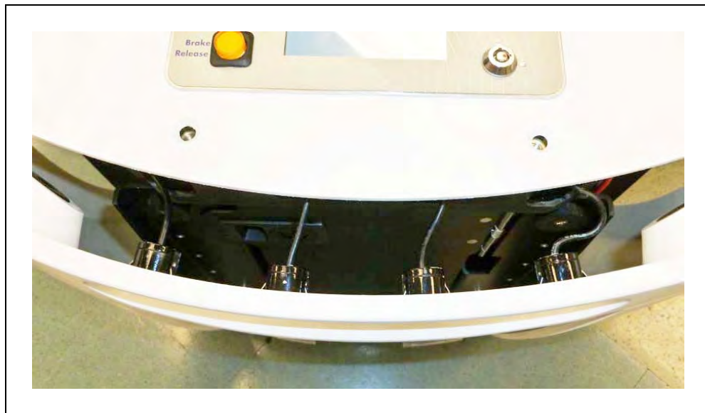
Figure 10-9. Sonar Leads, with Connectors Still in Chassis
