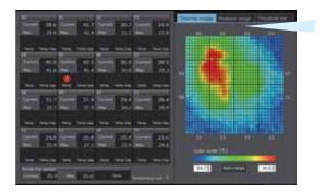
Confirm the temperature status by simultaneously displaying the temperature data and thermal image. Easily identify the device which is outputting an alarm.
