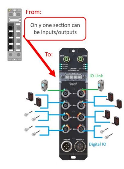
Each Port: Up to 1 IO-Link, 2 Digital Inputs, 2 Digital Outputs, or a mix
