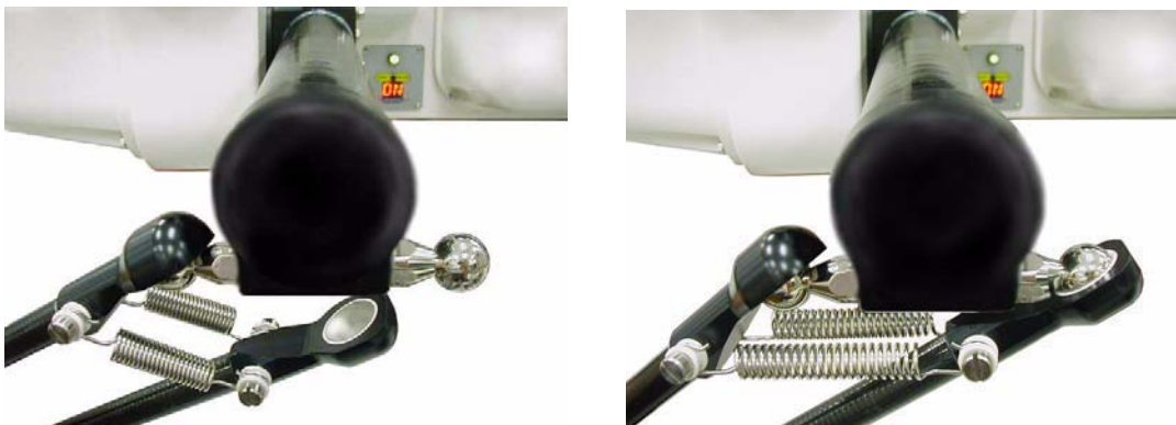
Figure 3-9. Installing Ball Joints
