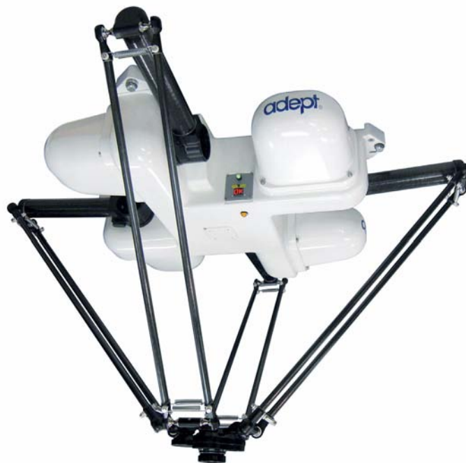
Figure 1-1. Adept Quattro s650H Robot
