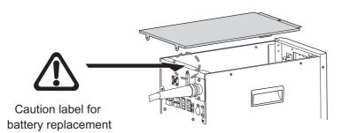
The caution label for battery replacement is attached to the top of the back plate and can only be seen when the lid opened.
