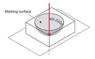
· Cone internal (X axis right vertex, Placed directly)
