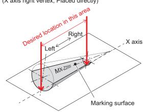
· Cone internal (X axis right vertex, Semi-cone)
