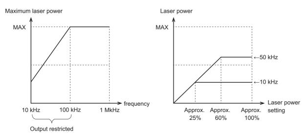
Graph showing restricted laser power when pulse pattern 1 is set
