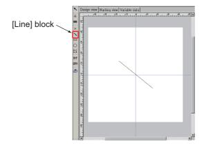
Mark a straight line from the specified start point to the end point (broken line can also be used).
