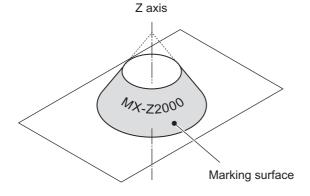
· Cone external (Y axis top vertex, Placed directly)
