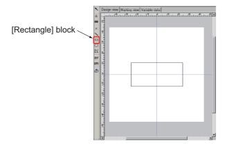
Mark a rectangle (box shape) (broken line can also be used).
