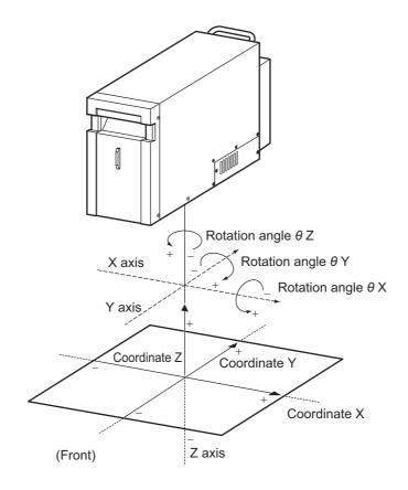
(Example) Rotation direction and tilt with a setting of  $\theta X = +$  direction, and  $\theta Y = +$  direction
