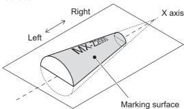
· Cone external (Y axis top vertex, Marking surface horizontal)
