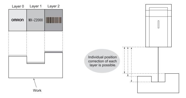
Also, for work with column, conical, and spherical shapes shown in the figure below, curved surfaces can also be marked by setting the work radius and number of divisions of the surface. Position correction is also possible for X, Y, Z axes and  $\theta$ Z.
