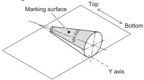
· Cone external (Y axis top vertex, Semi-cone)
