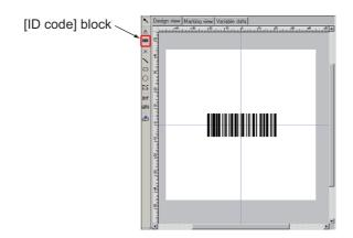
Mark a bar code or a 2D code. The following codes can be marked.
