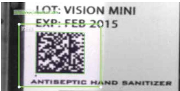
Reads a bar code or 2D code. The Match String function allows this smart camera to perform verification that is usually done by a PC or PLC.
