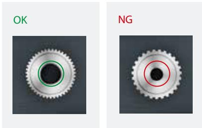
Orientation inspection of attached rubber
