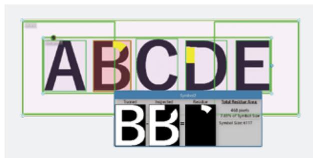
Detects defects from measured character strings using the registered reference character string. Automatically focuses on a target character string even if its position differs.
