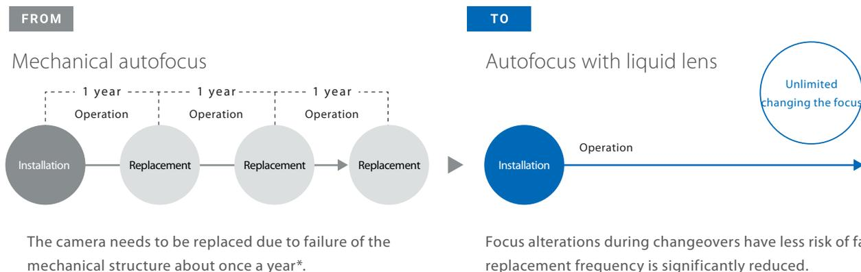
The F430-F/F420-F Series with a long-life liquid lens provides unlimited autofocus, easily focusing on different items just by switching the focus. The liquid lens greatly reduces the replacement frequency that is once every several months to several years with the mechanical autofocus lens.
