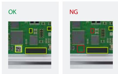
Presence inspection of PCB mounted components
