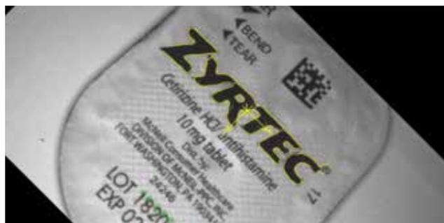
Outputs the position and angle of the registered image. The inspection area of this tool can automatically be used for the processing following this tool.
