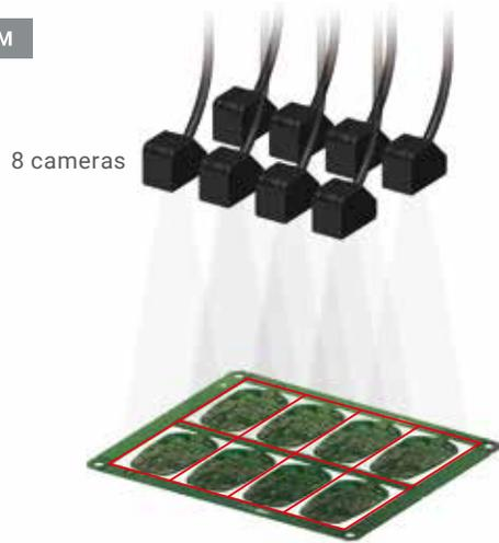
Mechanical design is required for multiple cameras. Positioning of the mechanism and fine-tuning of software are time consuming.
