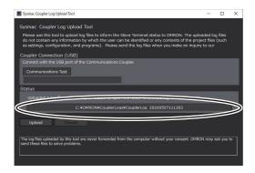
The log files are displayed in Windows Explorer. Send the log files to the support center.
