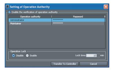
2 Select the Enable Option in the Operation Lock Area, enter the Lock time, and click the Transfer To Controller Button.
