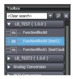
**2** Drag the library object to the ladder diagram. The function block from the library is inserted.
