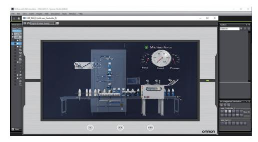
The Simulation Pane has a button that is used dedicatedly for simultaneous simulation of the Controller with an NA-series PT. Refer to *Dedicated Window for Simultaneous Simulation with NA-series PT* on page 7-117 for information on this pane.
