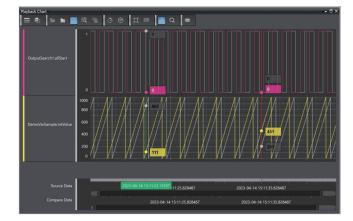
On the time series variable graph, the play position of playback data is indicated by the current time line.
