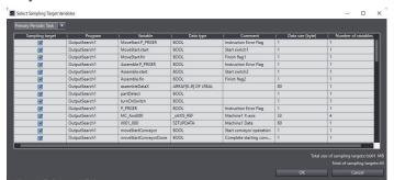
You can see the size of each variable in **Data size** column in the **Select Sampling Target Variables** dialog box. Sort by variable data size to see which variable has large data size.
