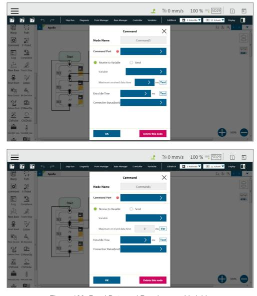
Figure 189: Read Data and Receive as a Variable
