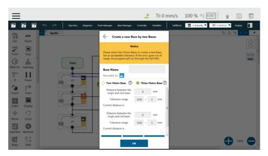
Figure 101: Create a New Base with Three Vision Bases
