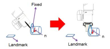
Figure 228: Base Coordinate System
