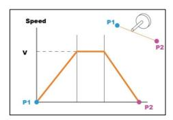
Figure 119: Speed of Line Motion
