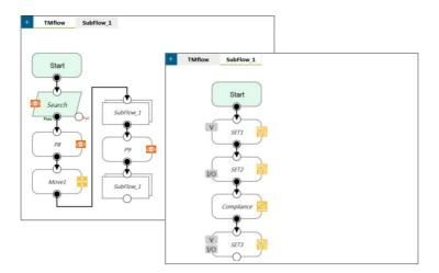
Figure 164: Subflow Node Modularization Concept
