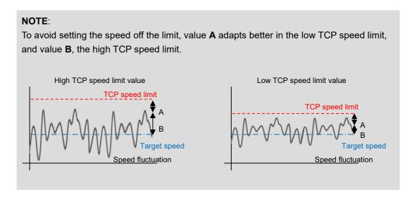
The custom values of the TCP speed and the Joint Speed are set in Setting>Safety>Performance Settings and Setting>Safety>Human-Machine Safety Settings>More Limit Setting for normal mode and collaborative mode, respectively.
