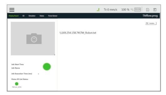
Figure 193: Display Node Displays Received Variables
