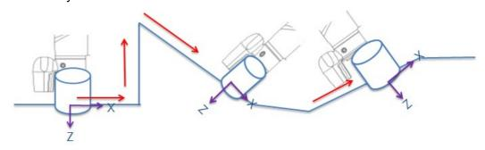
Figure 227: Tool Coordinate System
