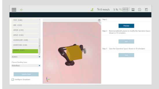
Users can select items named with (CAD) in the list at left as the operation space with the scenery file for the project. The actual position of the CAD in the scene will update as the dependent base updates. This is a great help for the collision check node to detect the collisions between the robot and the objects in the scene.
