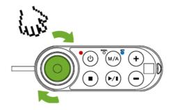
Figure 1: Release the Emergency Switch
