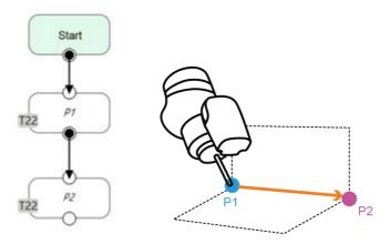
Figure 121: Line Application Example
