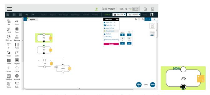
Figure 129: Speed Adjust and Speed Indication on the Node.
