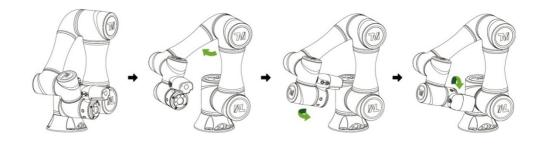
Figure 4: The Recommended Operating Sequence of Moving the Joints of TM Robot from Packing Pose to Safe Posture
