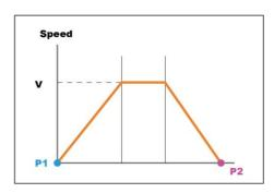
Figure 115: Speed of PTP Motion
