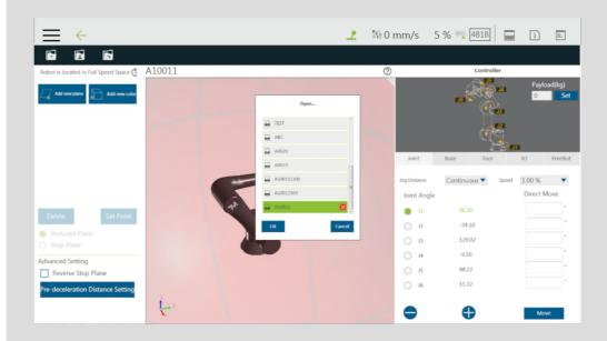
The icon before the file name denotes the operation space comes with the scenery file, and the object name and its dependent base will be shown at the top right of the 3D viewer when moving the mouse cursor on the object in the scenery file.
