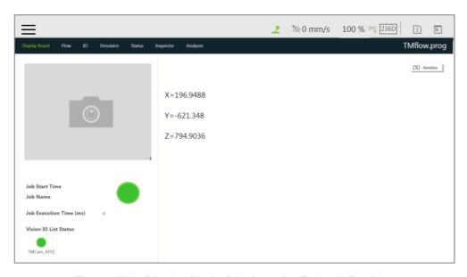
Figure 198: Display Node Displays the Robot's Position
