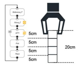
Figure 136: Plan for the Move Node
