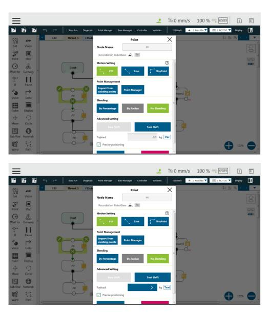
Figure 128: Motion Nodes Support Variable as the Inputs
