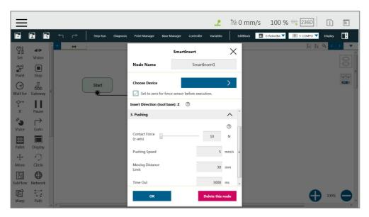
Figure 225: Pushing Parameter Interface
