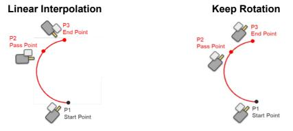
Figure 139: The Circle Motion Status of Reach End Point Setting
