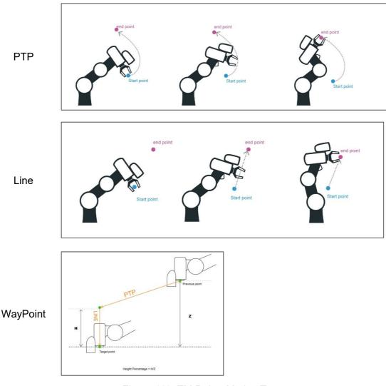
Figure 113: TM Robot Motion Types
