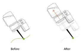
Figure 96: Tool Shift Using Keep Path
