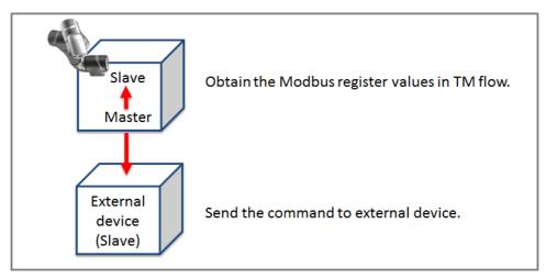
Figure 172: Robot Modbus Protocol
