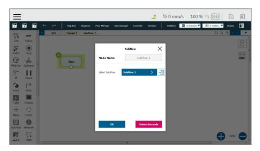
Figure 167: Select a subflow in the subflow node (2/2)
