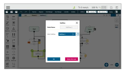
Figure 166: Select a subflow in the subflow node (1/2)
