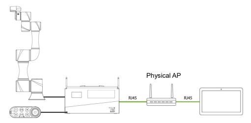
Figure 12: Wired Network Connection Method (1/2)
