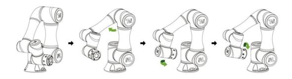
Figure 5: The Recommended Operating Sequence of Moving the Joints of X series
