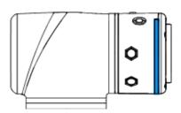
Figure 6: The Indication Light Ring of The End Module Returns to Blue Light
