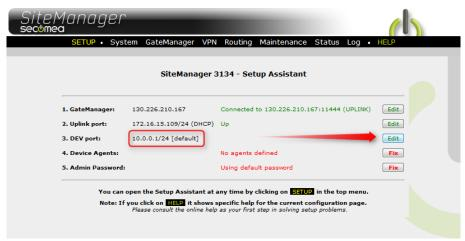
31. The PLC in our example has IP address 172.24.2.129/24 (/24 means it has subnet mask 255.255.255.0). So the address for the DEV port must be a free address in this subnet (172.24.2.x), for instance 172.24.2.128.
