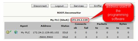
You now have IP access to the device from your PC through the LinkManager via the GateManager and SiteManager. You can therefore now connect directly to the IP address of the device using the native PLC software (in this example Siemens Step7 or the TIA portal).
