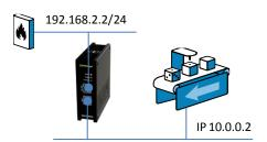
**HINT:** The machine depicted as 10.0.0.2, can be attached through a switch, or directly with an Ethernet cable to a **DEV** port. Optionally, the SiteManager can be configured to assign the address to the devices on the DEV ports by DHCP.
