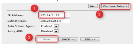
**Hint:** If your device is configured to receive an IP address from a DHCP server, you could have enabled DHCP in this menu, which would make the SiteManager act as a DHCP server that assigns IP addresses to devices on the DEV network.
