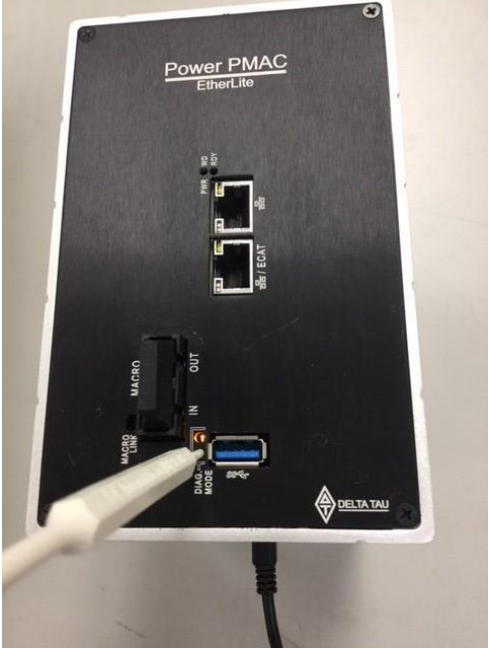
Figure 2. USB Connector is for a mass storage device
