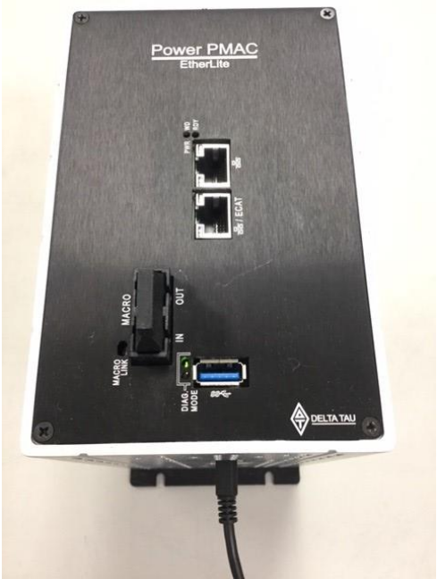
Figure 2. USB Connector is for a mass storage device
