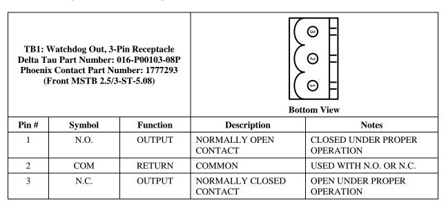
The TB1 connector provides the output signals for the watchdog timer circuit. It is recommended that this output be used as part of the safety circuitry for the system, so if the Power PMAC CPU loses power or trips its watchdog timer, the system will go into a safe shutdown mode without the assistance of any software on the Power PMAC CPU.
