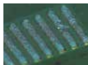
QFP Solder Shape (microscope)
