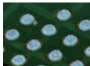
CSP Solder Shape (Shape Display VP6000M-V)
