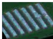
QFP Solder Shape (Shape Display VP6000M-V)
