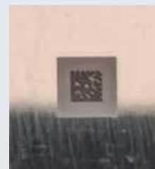
Aluminum buffing (mirror surface), with groundwork Cell size: 0.127mm
