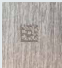
Aluminum hairline processing, unclear, no base processing Cell size: 0.127mm
