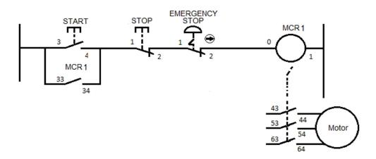
**Note:** This circuit using the G7SA can be used with a load that draws less than 6 Amps, if more than 6 amp load G7SA can be substituted with a J7 contactor to carry the load. If the circuit requires more emergency stops, add them in series with the circuit.
