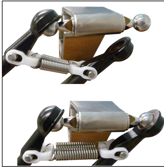
Figure 3-7. Pivot to Install Outer Arms
