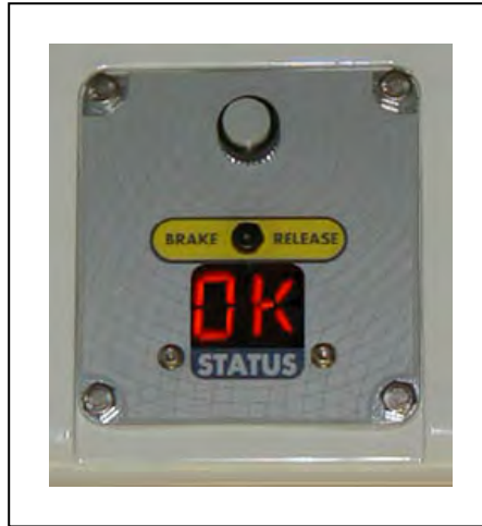
Figure 6-5. iX4-650H/800H Robot Status Panel
