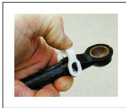
Figure 6-13. Push the retainer Into Position
