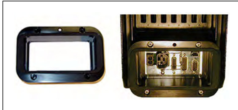
Figure 4-18. Cable Seal Housing (left), Installed (right)
