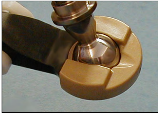
Figure 3-18. Ball Stud Lock in Correct Position
