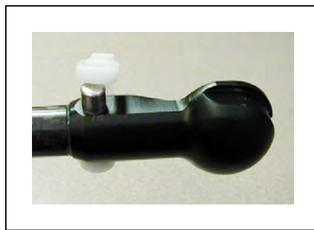
Figure 6-12. Retainer Over Top of Pin
