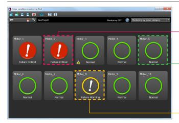
The conditions of up to 10 motors are displayed as a list through the K6CM Series connected to the network. The data of up to 30 K6CM units can be viewed. (Three types of K6CM can be installed to one motor)
