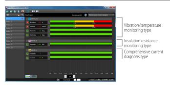
Displays the alarm statuses of multiple motors. Allows changes in the motor condition to be checked as a time series.
