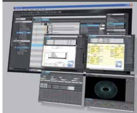
The Sysmac Studio IDE also reduces project time by allowing operators to test, debug, and simulate programs even before production hardware is in place. The software supports access through workstations, browsers, and mobile devices. Operators on the plant floor can also use an Omron NA series HMI to write and insert structured text directly into ladder programs.
