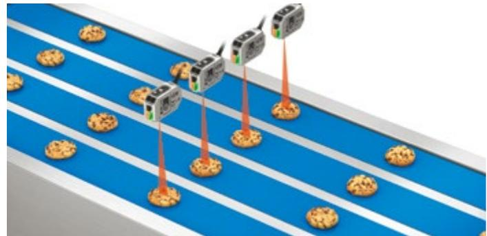
The mutual interference prevention function includes up to 4 units, allowing users to limit false detections when using multiple sensors on the same line.
