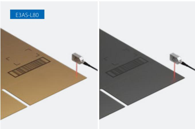
Detection may become unstable as differential travel varies depending on the target color. The E3AS-L80 Sensor can reliably detect level difference regardless of color since its differential travel<sup>2</sup> for black paper is 5%.
