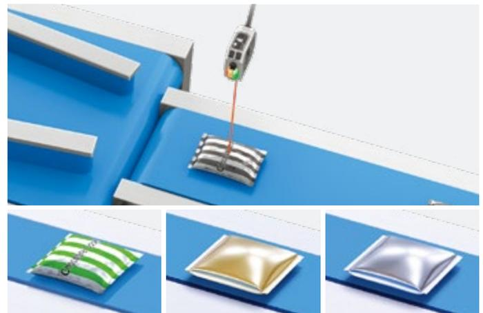
Surface variation causes unreliable light reception back to the sensor with a spot beam. The E3AS-HL line beam minimizes the impact of the surface profile by reflecting off more surface area.
