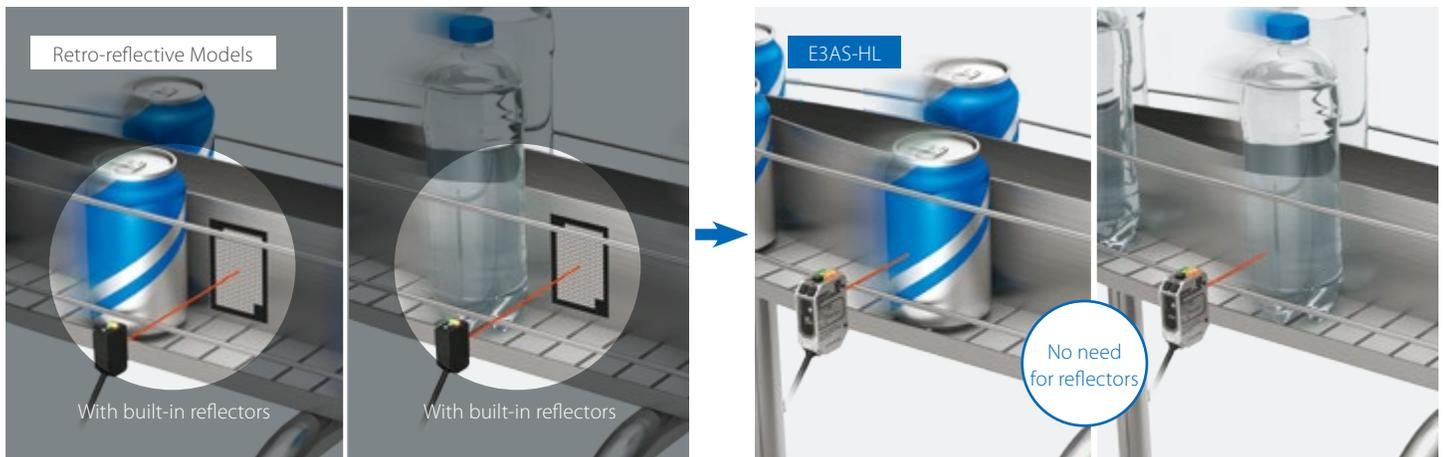
Retro-reflective sensors are used to detect curved surfaces of cans and transparent plastic bottles, but present installation issues when mounting reflectors on multi-lane conveyors.
