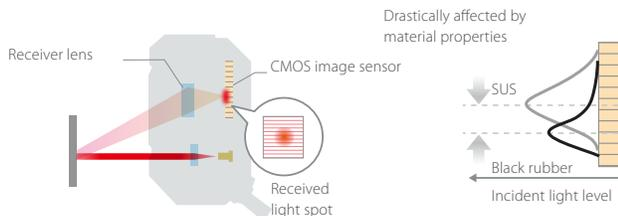
**To** Material properties minimally affect detection because the receiver lens position is automatically adjusted to the micrometer level to minimize the received light spot.
