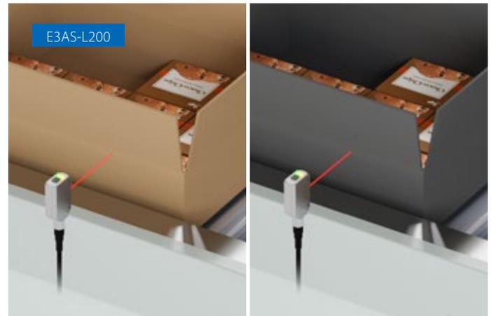
When the target is low-reflective black paper, detection may become unstable due to insufficient sensing distance. The E3AS-L200 Sensor can stably detect at the same distance regardless of color since its sensing distance for both white paper and black paper is 200 mm.
