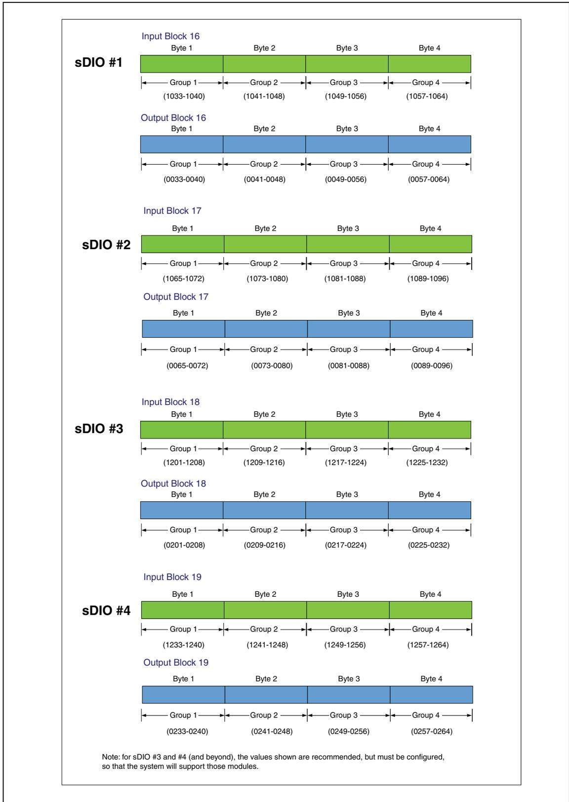
Figure 7-8. Input/Output Block Configuration for Optional sDIO Modules
