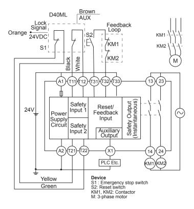
D40ML to G9SE-201 - Series Connections (up to Safety PLd acc. EN ISO 13849-1, maximum 20 switches)
