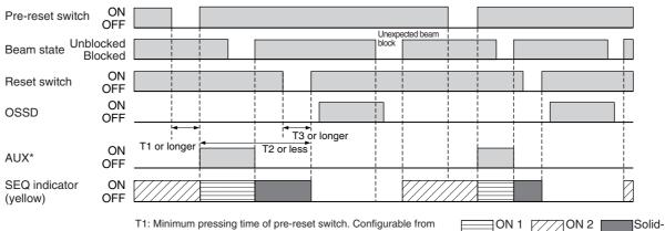
11: Minimum pressing time of pre-reset switch. Configurable from 100 to 500 ms in 100-ms increments. T3 = T1
