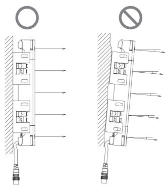
Mounted on a level, flat surface.
