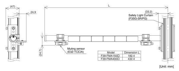
Mounting F39-FMA□□□□-R on Floor Mounting Column (F39-ST□□□□)
