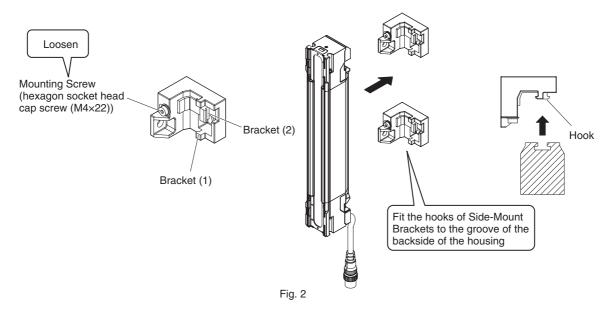
**3.** Securely tighten the Mounting Screws to fix the Side-Mount Bracket to the sensor housing. The recommended torque to tighten the Mounting Screws is 3.0 N•m. Then loosen the Alignment Screws (Fig. 3)
