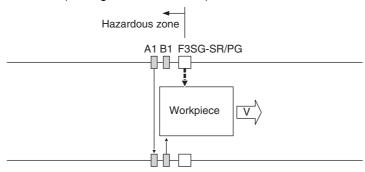
The workpiece has completely passed the muting sensor A1 and the sensor is now in the OFF state. In the Standard Muting mode, the Muting state is released here. In the Exit-Only Muting mode, the F3SG-SR/PG's safety function is disabled for the exit-only muting delay time: T5.
