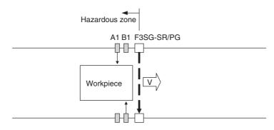
When the muting sensors A1 and B1 are turned ON in this order, and the MUTING state is enabled. In this state, the safety function of F3SG-SR/PG is disabled.
