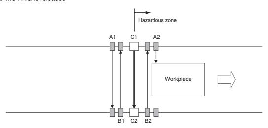
The muting sensor B2 is turned OFF, the Muting state is released, and the safety function of the F3SG-SR/PG C1 and C2 is enabled.
