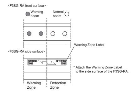
When the warning zone is enabled, the CFG indicator of the F3SG-SR receiver turns ON.
