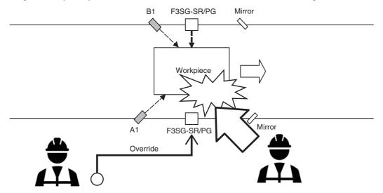
Install the F3SG-SR/PG so that it is not affected by reflective surfaces. Failure to do so may hinder detection, resulting in serious injury. For an installation distance from reflective surfaces, see *5-1-3. Distance from Reflective Surfaces*.
