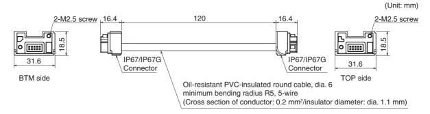
Side-by-side Cascading Cable for Receiver
