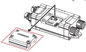
**4.** Set the DIP-SW channels 1 to 8 OFF of the new intelligent tap to attach.
