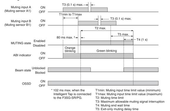
Note. This timing chart shows the case in which the MUTING state was released under the condition of T4 (1 s).
