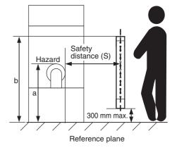
Note: Lower edge of the detection zone above 300 mm in relation to the reference plane does not offer sufficient protection against crawling below.
