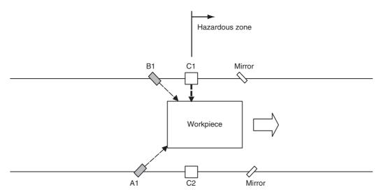
The F3SG-SR/PG C1 and C2 are blocked but the safety function is disabled due to MUTING, and the OSSD 1 and 2 are turned ON.
