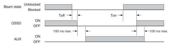
Ton: OFF to ON response time Toff: ON to OFF response time
