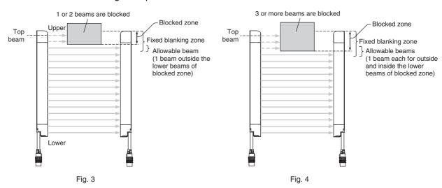
• When beams are blocked within the range from [1 beam next to bottom beam] to [1 beam next to top beam] When beams are blocked within the range from [1 beam next to bottom beam] to [1 beam next to top beam], allowable beams are configured as follows.
