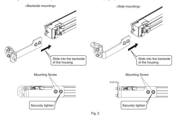
Tightening screws with a torque that considerably exceeds the recommended torque may cause failure.
