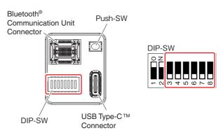
For details of the channels, refer to 3-5. DIP Switch on Intelligent Tap.
