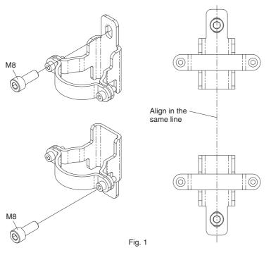
Screws to mount the brackets to the wall are not included.
