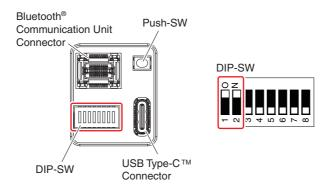
**4.** Set the DIP-SW channels 3 to 8 ON or OFF as needed.
