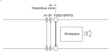
A workpiece has passed the F3SG-SR/PG's detection zone. When the muting end wait time: T4 (1 s: configurable) passes after the F3SG-SR/PG is unblocked, the MUTING state is released.
