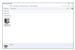
**4.** When selecting the [Hardware] tab, the screen below is displayed that indicates a COM port. In this example, the device "000000001\_F3SG-4SRA0160-25" is set to COM7.
