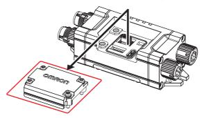
3. Set the DIP-SW channels 1 and 2 ON.
