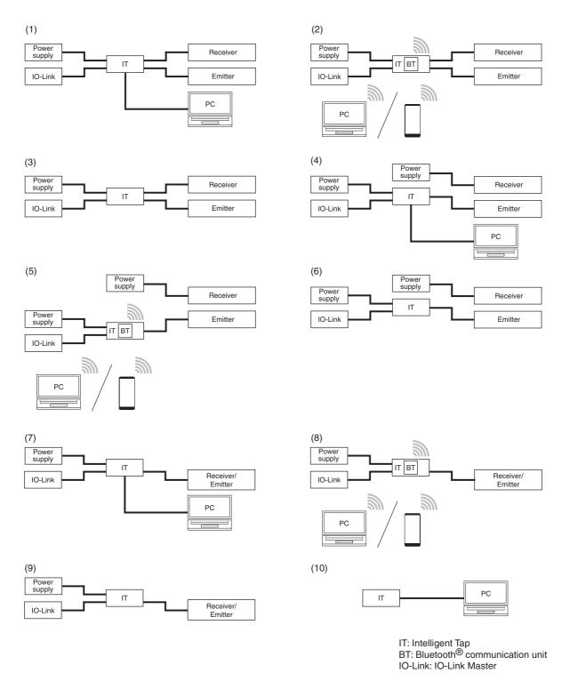
For the patterns (1), (4) and (7), turn the power on and start the SD Manager 3 on the PC. For the pattern (10), the power is supplied from the PC to the Intelligent Tap.
