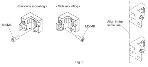
Screws to mount the brackets to the wall are not included.
