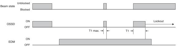
T1: Allowable delay time. This parameter can be set by 0.1 s in a range of 0.1 to 4.0 s.
