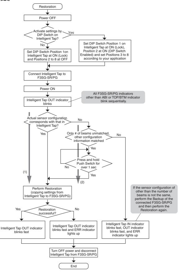
If the sensor configuration (model and cascading) in the Intelligent Tap corresponds with that of the actual one, the Restoration is automatically performed.(1)
