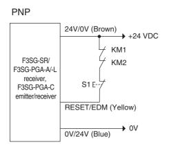
S1: Lockout or interlock reset switch KM1, KM2: External device
