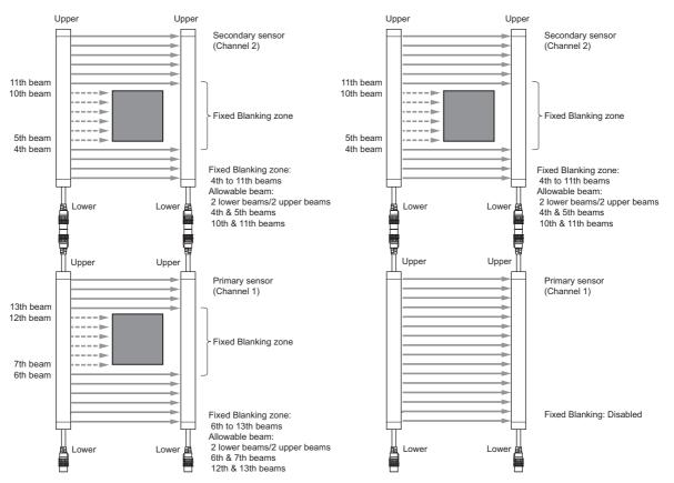
• The Teach-in result for Fixed Blanking and Floating Blanking cannot be saved together. When the Teach-in is ferformed for Floating Blanking, the result of the Teach-in for Fixed Blanking is cleared.
