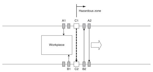
When the muting sensors A1 and B1 are turned ON in this order, MUTING starts. In this state, the safety function of F3SG-SR/PG C1 and C2 is disabled.
