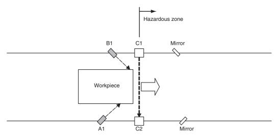
When the muting sensors A1 and B1 are turned ON in this order, the F3SG-SR enters the MUTING state. In this state, the safety function of F3SG-SR/PG C1 and C2 is disabled.
