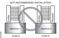
In the Wired Synchronization, mutual interference is prevented in up to 3 sets, using interference light avoidance algorithm.
