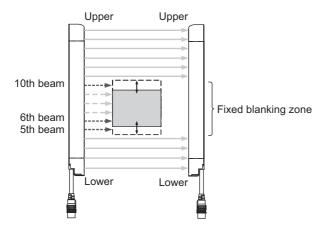
When a fixed blanking zone is configured by the Teach-in with the Push Switch or the Muting Input A, the fixed blanking zone and allowable beams are configured automatically depending on the position of blocked beams and the following conditions.
