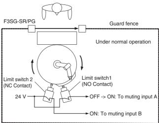
Rotation of a robot arm sets the muting input A from OFF to ON. The safety function of the F3SG-SR/PG is enabled.
