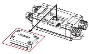
**4.** Set the DIP-SW channels 1 and 2 ON of the new intelligent tap to attach.
