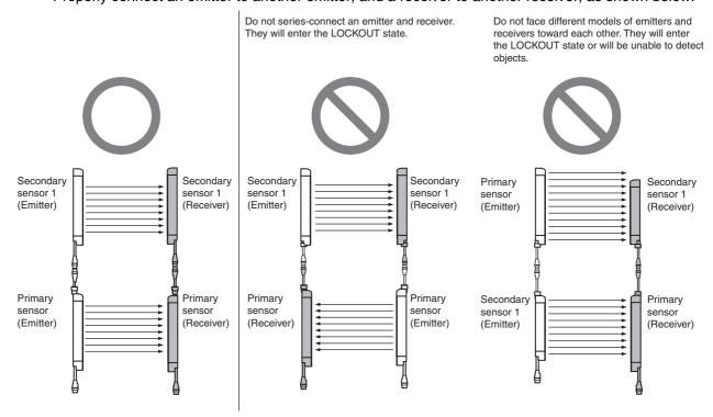
·(e) If caps and Cascading Cables are not connected properly, the F3SG-SR enters lockout (when power is turned ON). CHECK!
