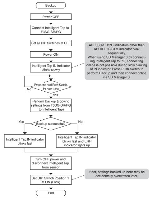
To run the Intelligent Tap while being connected to the F3SG-SR/PG, you must save the F3SG-SR/ PG's settings in the Intelligent Tap by the backup operation. After performing the Backup, set the DIP Switch Position 1 at ON (Lock) and connect the Intelligent Tap to the F3SG-SR/PG.
