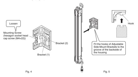
5. Securely tighten the Mounting Screw to fix the Adjustable Side-Mount Bracket to the sensor housing. The recommended torque to tighten the Mounting Screw of the Adjustable Side-Mount Bracket is 3.0 N•m. Then loosen the Alignment Screw (hexagon socket head cap screw (M4×22)) of the Adjustable Side-Mount Bracket. (Fig. 6)
