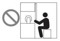
While working, a person is inside the sensor's detection zone.
