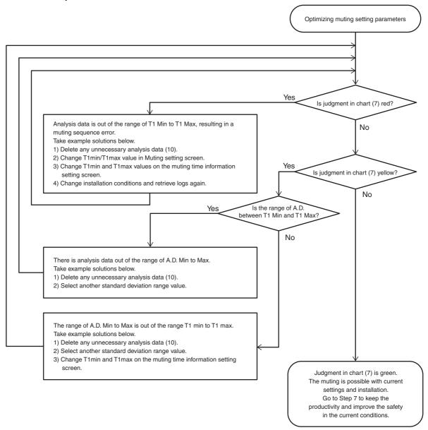
7. Adjusting the T1 Min and T1 Max closer to the A.D. Min and Max allows the user to keep the productivity and improve the safety.
