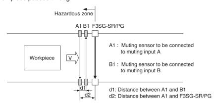
All muting sensors are turned OFF and the safety function of the F3SG-SR/PG is working.
