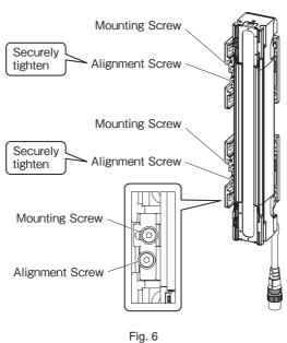
Tightening screws with a torque that considerably exceeds the recommended torque may cause failure.
