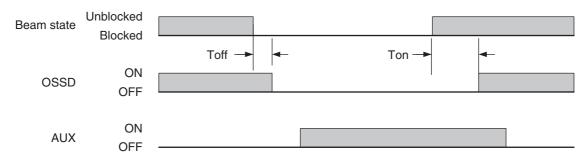
Ton: OFF to ON response time Toff: ON to OFF response time
