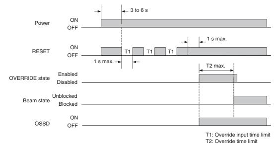
Note. In this timing chart, the OVERRIDE state ends when the F3SG-SR/PG receives light.
