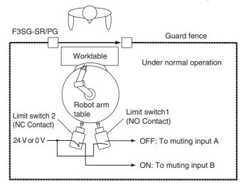
The safety functions of the F3SG-SR/PG is activated with the limit switch 1 being in OFF and the limit switch 2 being ON.
