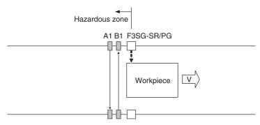
The workpiece has completely passed the muting sensor B1 and the sensor is turned OFF. The F3SG-SR/PG disables its safety function if it is within the exit-only muting delay time.
