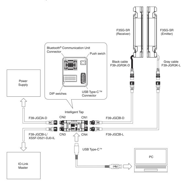
For F3SG-SR-K, use a terminal block to connect to an intelligent tap as it is the open-ended type. The figure below shows a connection example of F3SG-SR-K and the intelligent tap.
