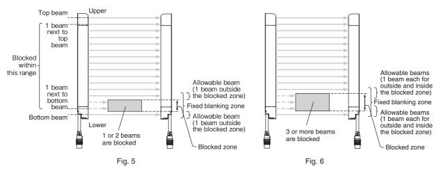
The table below lists the number of allowable beams when a fixed blanking zone and allowable beams are configured with the SD Manager 3.
