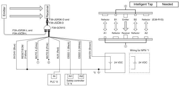
PLC: Programmable logic controller (Used for monitoring only. NOT related to safety system.) A1, A2, B1, B2: Muting sensor (E3Z-R□6)
