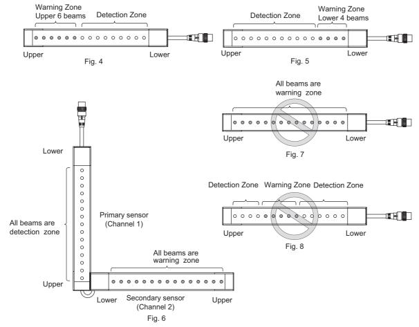
When a warning zone is configured, you must attach Warning Zone Label (included) that indicate a border between normal detection zone and warning zone.
