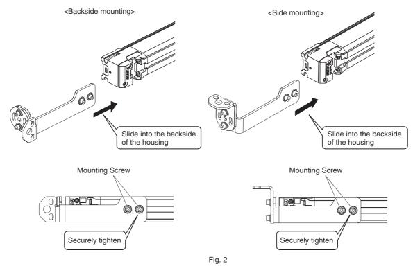
Tightening screws with a torque that considerably exceeds the recommended torque may cause failure.
