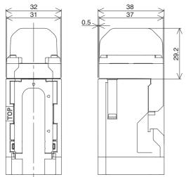
Material: PC resin (Transparent cover) PBT resin (Base)
