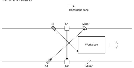
The muting sensor A1 is turned OFF, the Muting state is released, and the safety function of the F3SG-SR/PG C1 and C2 is enabled.
