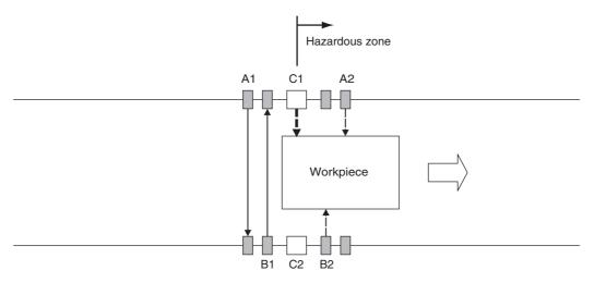
The muting sensors A1 and B1 are turned OFF but A2 and B2 are ON, so the MUTING state is still maintained. The OSSD 1 and 2 are turned ON.
