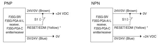
S1: Lockout or interlock reset switch
