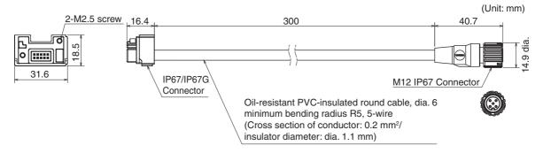
Receiver Cascading Cable for Extended
