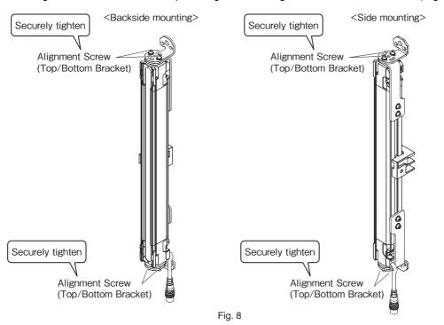
Tightening screws with a torque that considerably exceeds the recommended torque may cause failure.
