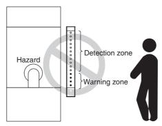
A warning zone must be configured based on a safety distance.
