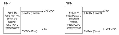
The F3SG-SR is set to PNP when the 24V/0V line (brown) is connected to +24 VDC and the 0V/24V line (blue) to 0 V.
