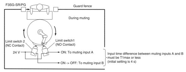
If the duration between when the muting input A is turned ON from the OFF state and when the muting input B is turned OFF from the ON state is within T1max [s], the safety function of the F3SG-SR/PG is disabled.
