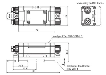
Material: PBT resin (Body parts) [Unit: mm]
