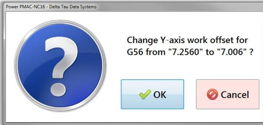
The PPNC software always highlight the current active work offset in a table. If no work offset is active or it is desired to change another work offset beside the one is active, highlight it by clicking on it and then use automatic work offset buttons to set any or all positions.
