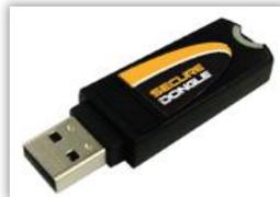
The hardware key is compatible with all versions of Windows and does not require a driver to be pre-installed.
