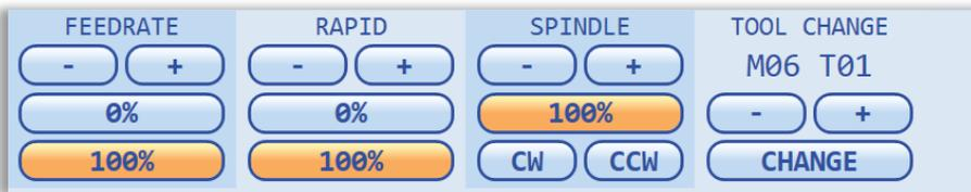
The soft panel is used to display and change Feedrate Override, Spindle Override, as well as control tool changes. If hardware control panel is presented, by default soft panel only shows the status of its members only such as zero or hundred percent override. If hardware control panel is not presented, soft panel can be used to show status as well as
