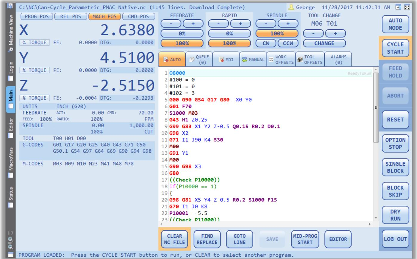
Full Screen mode will extend the PPNC to the video resolution boundaries. The Windows task bar will be covered by the bottom portion of the PPNC application. The operator can either use the Window button or ALT-TAB to move to other applications if desired. If Full Screen mode is selected it will be retained through application shut down.
