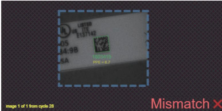
With nothing currently registered as the Master Symbol, when a Read is executed with Matchcode ON, the result is *Mismatch*.
