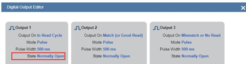
Advanced Settings: I/O - Output 1 - 3 Parameters - Output State
