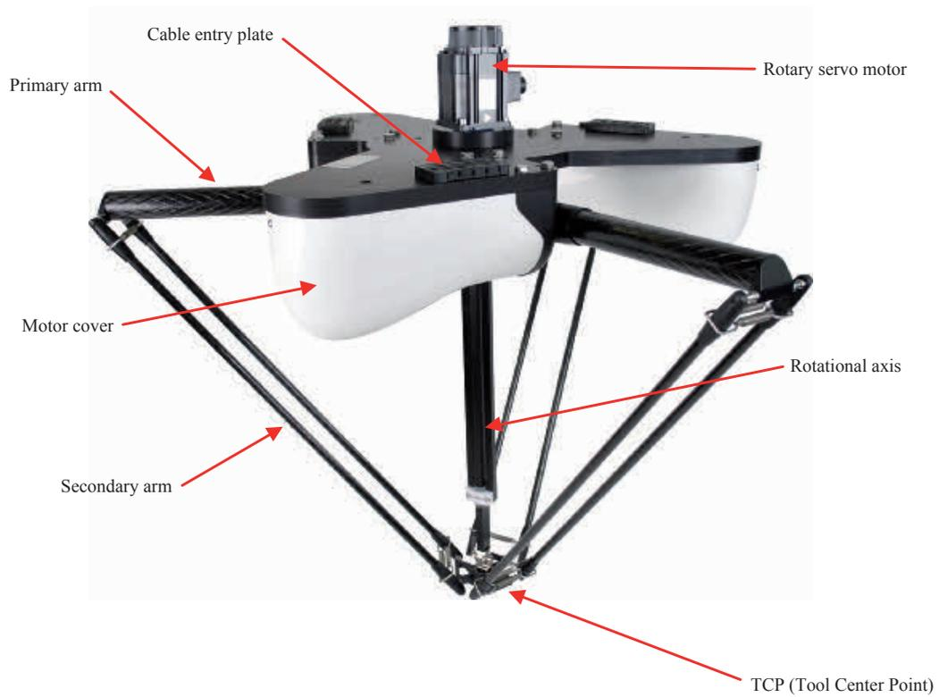
The CR\_UGD4\_XL robot consists of three radially placed axis which give the TCP freedom to move in three directions, X, Y and Z. An optional fourth axis can take care of the rotation,  $R_z$ , of the TCP.
