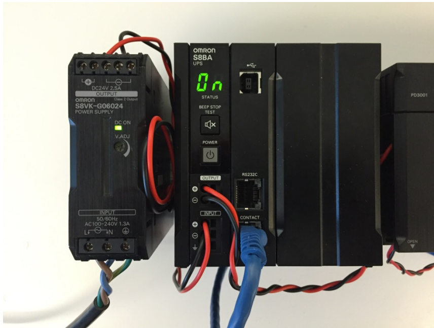
Figure 2 – Wiring of S8VK to S8BA
