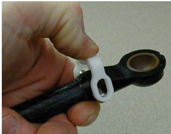
Figure 9-14. Squeezing the Horseshoe into Position
