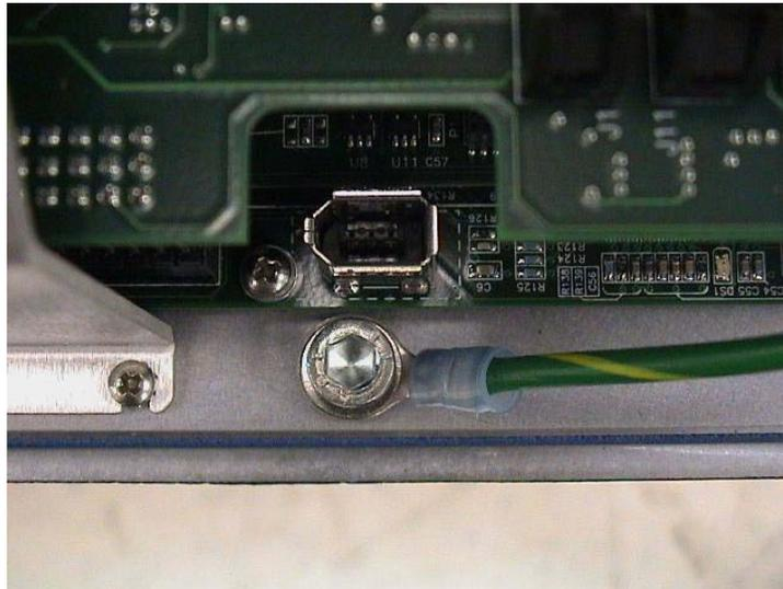
Figure 9-3. Ground Screw on AIB Chassis
