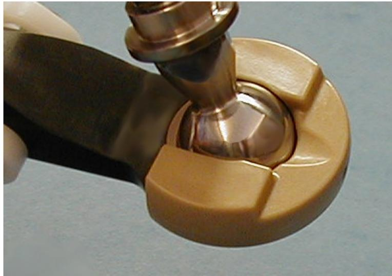
Figure 6-2. Ball Stud Lock on Ball Joint Socket
