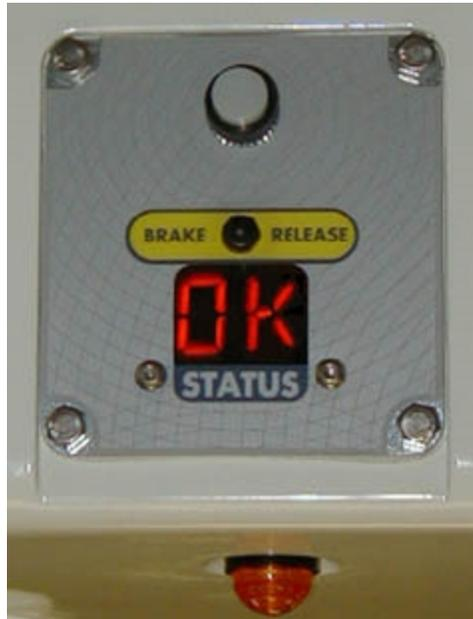
Figure 8-8. Status Display Panel, Showing 4 hex-head Bolts
