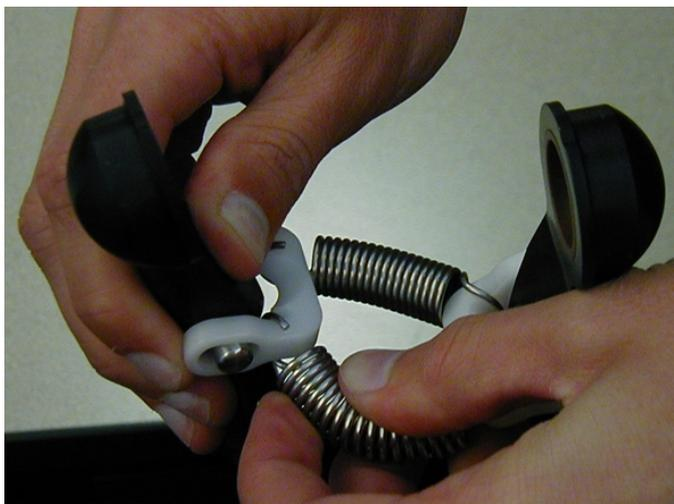
*Figure 8-10. Removing an Outer Arm Spring*
