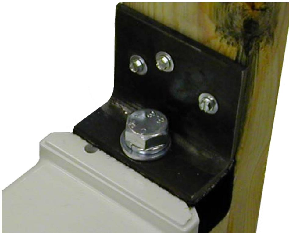
Figure 3-3. L-Bracket Securing Robot to Shipping Crate
