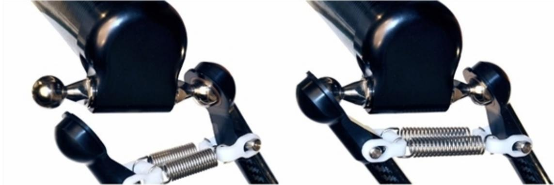
Figure 3-20. Installing Ball Joints (Quattro H shown)
