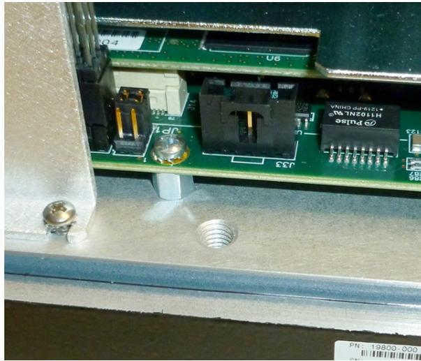
Figure 8-5. Cable Ground Screw Hole on eAIB Chassis
