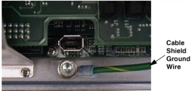
Figure 8-4. Cable Ground Screw on AIB Chassis
