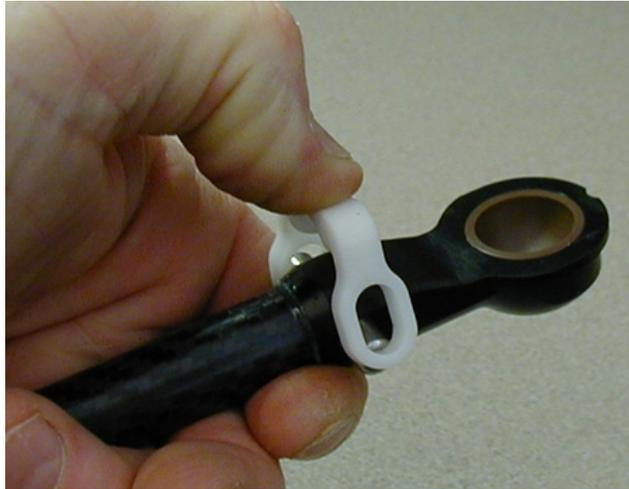
*Figure 8-14. Squeezing the Horseshoe into Position*
