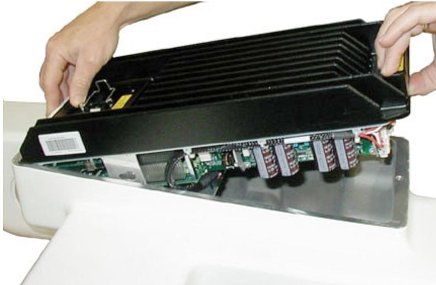
Figure 8-2. Opening the Chassis
