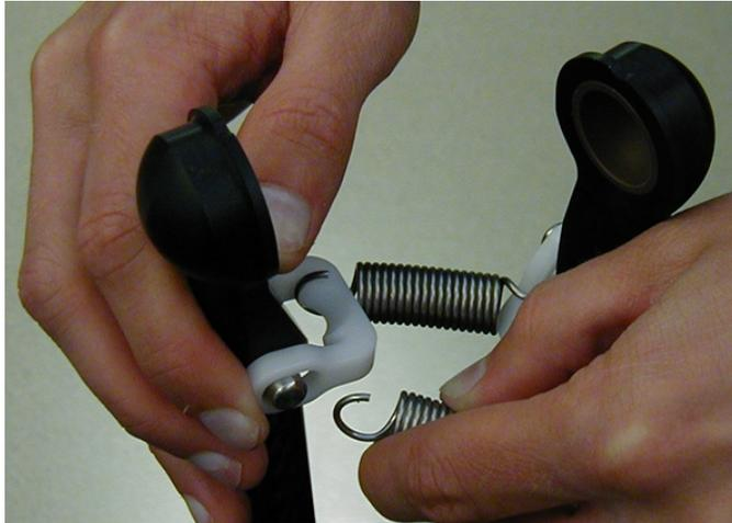
*Figure 8-11. Spring, with End Removed from Horseshoe*
