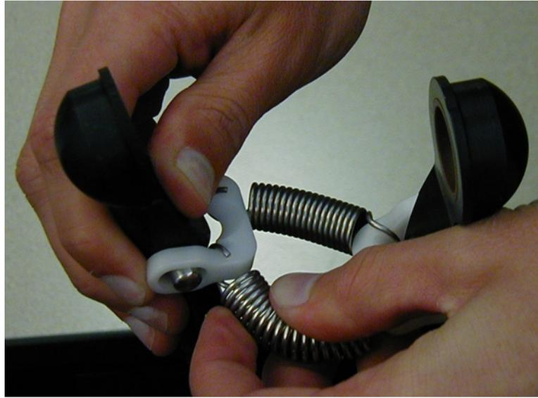
Figure 9-10. Removing an Outer Arm Spring
