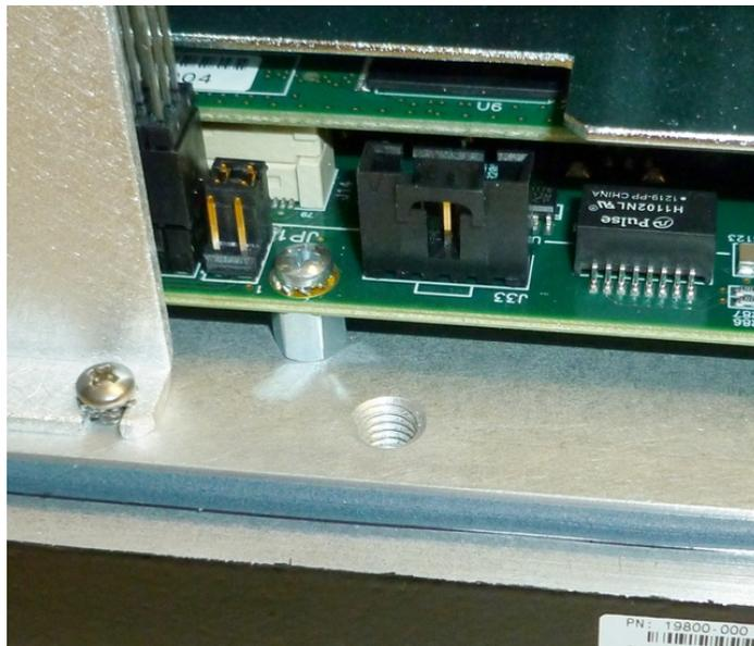
Figure 9-4. Ground Screw Hole on eAIB Chassis
