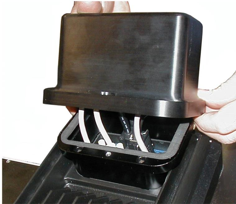
*Figure 10-10. Installing Cable Entry Top Cover Assembly*
